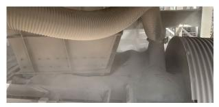
The excessive dust not only posed environmental and health risks but also increased operational costs due to the need for secondary dust control measures such as conveyor covers, active dust extraction, sealing, and water addition. Seeking a more effective and sustainable solution, the client engaged EMtek to redesign the chute using advanced simulation techniques.
